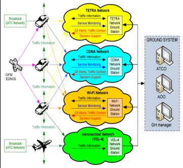
AIRNET platform will enable the elaboration of airport situation by real-time acquisition of aircraft and vehicles position through a set of wireless networks. The performances and the reliability of the wireless communication network is a key driver to the "end-to-end" quality of service.
