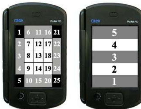
Figure 2. QTEK 9000. Screen positions (left): white – middle; gray and black: edges. Vertical distances (right).
