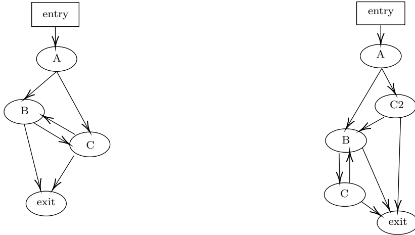
Figure 3.21: Node splitting technique applied on the graph on the left results in the graph on the right.
