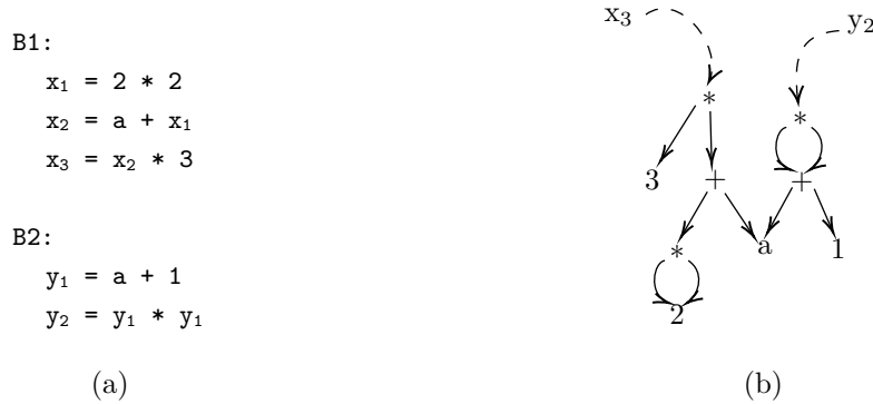
Figure 2.8: Shared value graph on the right (b) with the corresponding code on the left (a), where B1 and B2 are two different basic blocks. The shown instructions are not written in any specific programming language.
