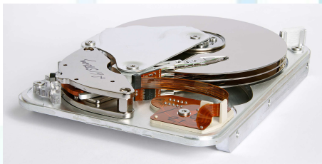
Figure: Interior of a magnetic hard drive
