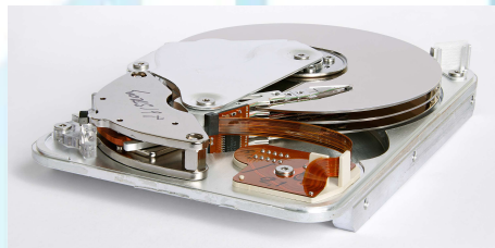
Figure: Interior of a magnetic hard drive
