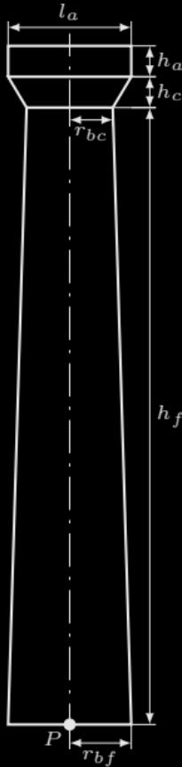
**column**( $p, h_f, r_{bf}, h_c, r_{bc}, h_a, l_a$ ) =
