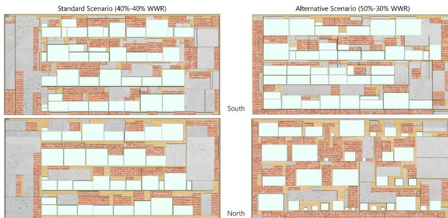
Fig. 8. Best packing configurations achieved in experiment 1 for scenarios 1 (40-40 WWR) and 2 (50-30 WWR): light blue represents the reused windows, textured grey represents concrete panels, the brick texture illustrates the brick panels, and the wood texture indicates the use of new wood cladding.
