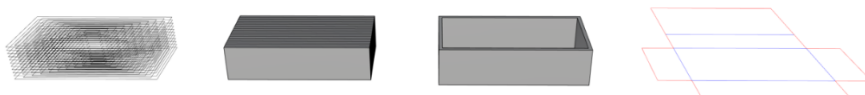
Fig 7. Automatic production of technical documentation for the same shape according to the selected manufacturing technique: 3D printing, sectioning, casting, and laser cutting.
