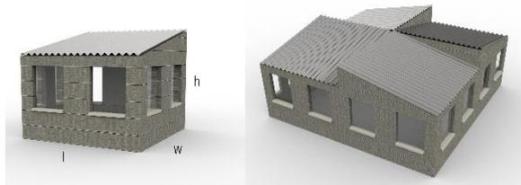
Fig. 4 – Unit parameters (left) and  $n = 4$  units (right).
