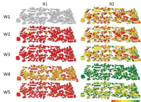
Fig. 7 – Heatmap of increase in thermal autonomy (%), compared to the zinc scenario and roof 1 (in grey).
