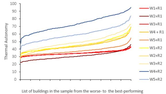
Fig. 6 – Thermal Autonomy from worse to best performing house for each construction scenario (comfort spectrum).
