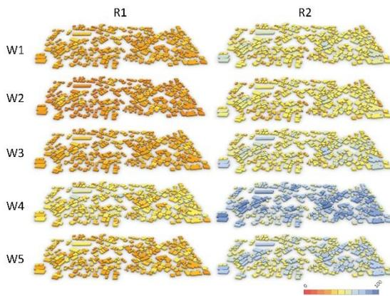
Fig. 5 – Chamanculo C thermal autonomy 3d model heatmap for the different construction scenarios
