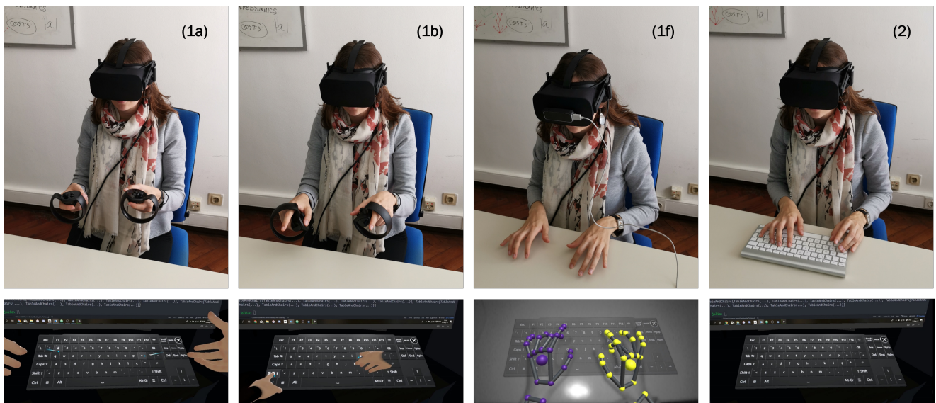
Figure 8. Tested typing options with corresponding visual feedback in VR below: virtual keyboard - wearing the control handles using (1a) laser tags, (1b) index fingers only, or (1f) leap motion technology; and (2) occluded physical keyboard, with a corresponding virtual keyboard with highlighted keys.
