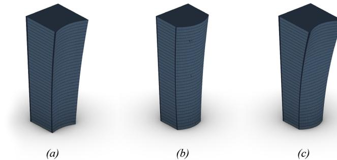
Figure 3. Design variations for the case study geometry: (a) original design, with a concave façade; (b) convex façade; (c) concave and convex façade.
