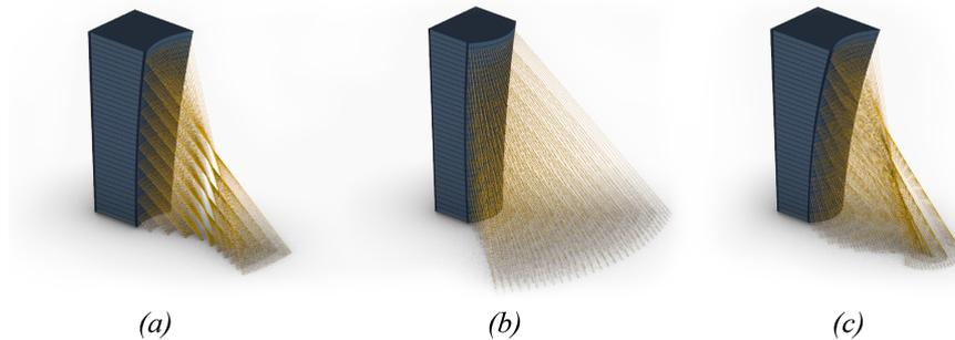
Figure 5. Preliminary feedback for the reflection of sun rays in the three building variations.
