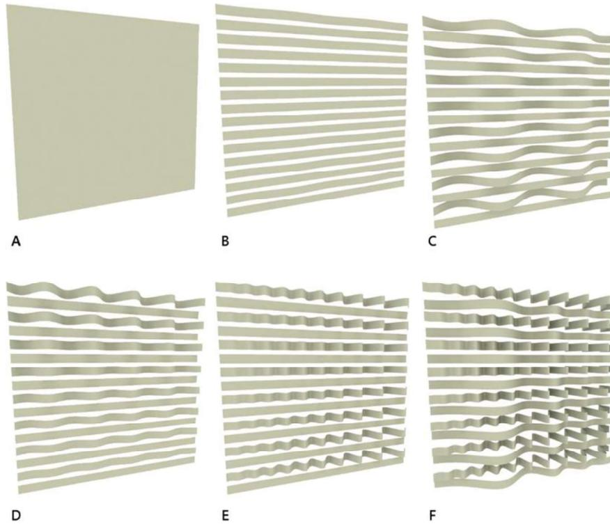
**Fig. 3.** The application of both *stripe* and  $T_{bend}$  functions: A. The initial surface; B. Creation of  $n$  horizontal stripes; C.  $T_{bend}$  algorithm with one transformation; D. Amplitude increasing with the vertical direction; E. Amplitude increasing with the horizontal direction; F.  $T_{bend}$  algorithm with two transformations.
