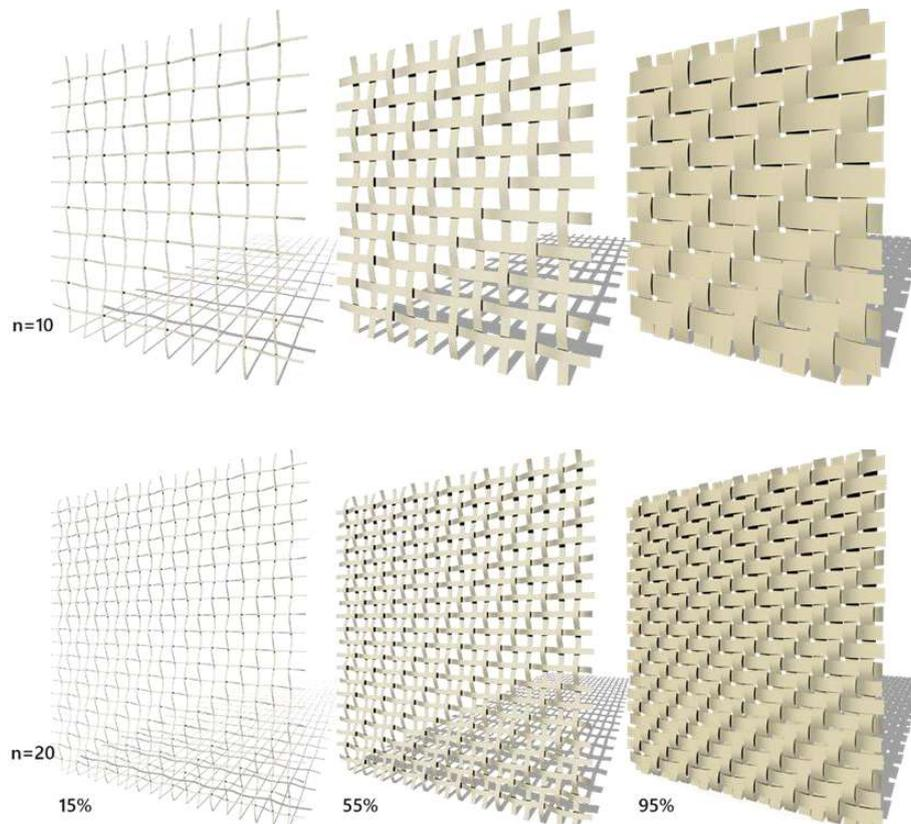
**Fig. 11.** A set of optimized weaving patterns: the top solutions have 10×10 stripes and the bottom ones have 20×20 stripes, and each column matches a percentage of opaque area - 15%, 55%, and 95%, correspondingly.
