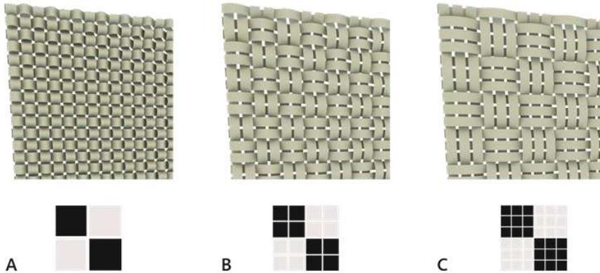
**Fig. 7.** Three weaving patterns available in the GS: A. chess, B. double-chess, and C. triple-chess.
