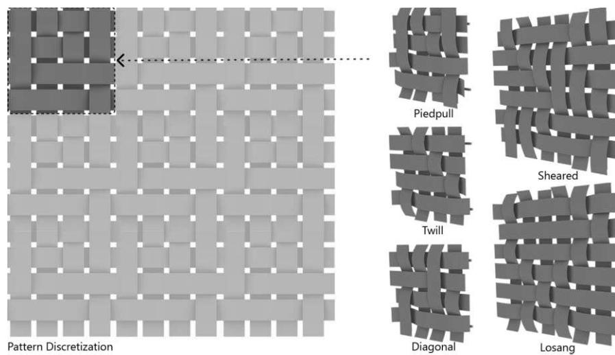
**Fig. 12.** Left: Discretization process of a façade weaving pattern based on a *piepull* pattern; Right: a set of different façade modules resulting from different weaving patterns.
