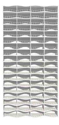
Fig. 1. On the right: An instance of the model inspired in the Marriott Hotel in Anaheim, which was totally implemented using Processing. On the left: the development stages. The sine curves defined (A) the slabs' shape, (B) the geometry of the guards, i.e. the handrails and the placement of the vertical elements (cylinders), and (C) the shape of the division walls. Source: Authors' own work.
