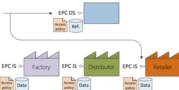
Figure 16: EPC Network architecture with DS and IS and security policies.
