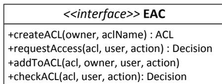
Figure 10: EAC interface operations.
