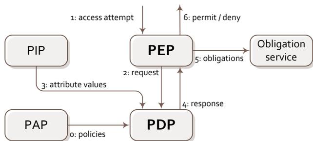
Figure 5: XACML request processing.
