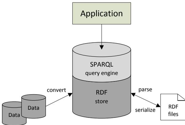
**Figure. 7:** Linked Data application architecture, adapted from [26].
