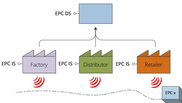
Figure 1: EPC Network architecture with DS and IS.
