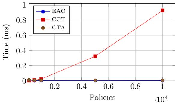
**Figure 17:** Raw evaluation time with increasing number of policies.
