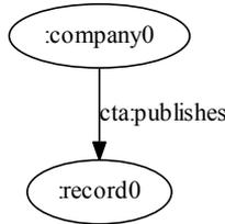
**Figure. 6:** RDF triple represented as a graph.
