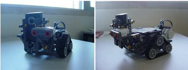
Fig. 2 Prototype mobile robot with a smartphone.
