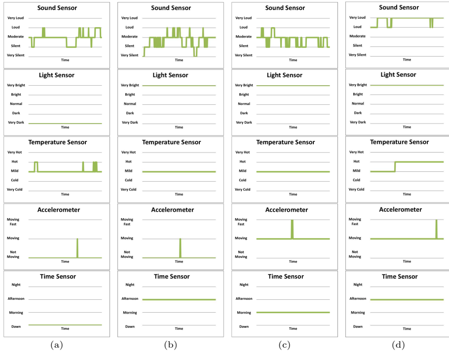
Fig. 5. Sensor readings for different contexts: sleeping (a), working (b), exercising (c) and driving (d).
