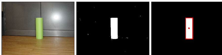
Fig. 3. Image captured with a green landmark (left image); Binary image after the application of the color segmentation (middle image) and landmark boundary detection after the application of the image noise reduction filter (right image).
