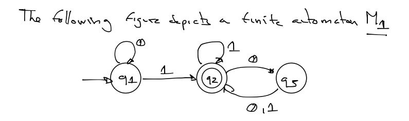
Formal definition of a finite automation Q: So what is the formal Sectiniton of an automate? A finite actomation has everal purk: - Set of states and reles for going from one state to another depending on the inpt symbol; - An input alphabet that indicates the allowed impet symbols; \_ It has a start state and a set of final states - A finite actumeton is a list of these
