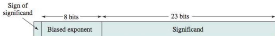
Figure: Typical 32-Bit floating-point format (Source: (Stallings, 2015))
