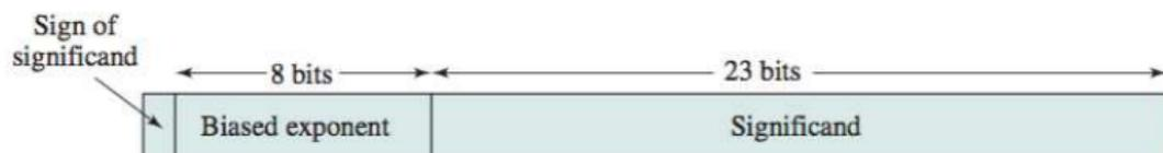
Figure: Typical 32-Bit floating-point format (Source: (Stallings, 2015))
