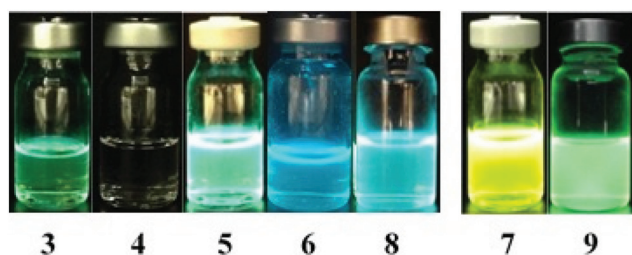
Fig. 6 Fluorescence colours displayed by complexes 3–9 in THF under UV-irradiation at 365 nm.
