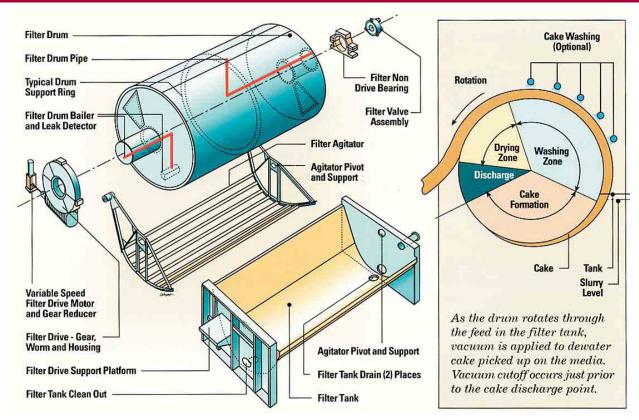
Our Drum Filters provide high filtration rates and have excellent washing characteristics. Wide variations are possible in cycle time to ensure optimum cake formation, dewatering and washing on any flowsheet. Our drum filters are ideally suited for filtering solids when a uniform deposit of cake on the media is desired, or when the cake is difficult to discharge.
