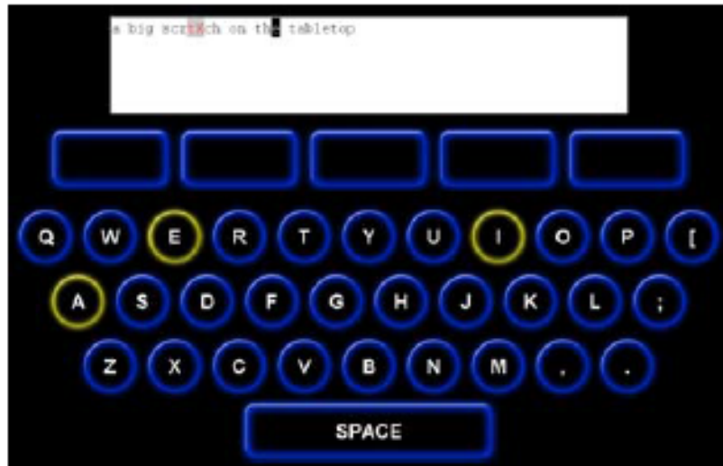
Figure 3.8: On-screen keyboard with letter prediction, highlighting "a", "e" and "i" keys.
