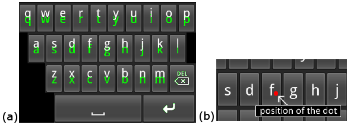
Figure 3.5: (a) The two different positions of the keys' labels. The green labels show the default Android keyboard and the white labels show the elevated labels; (b) keyboard that shows a red dot at the position where the user touches the screen after typing an "f".
