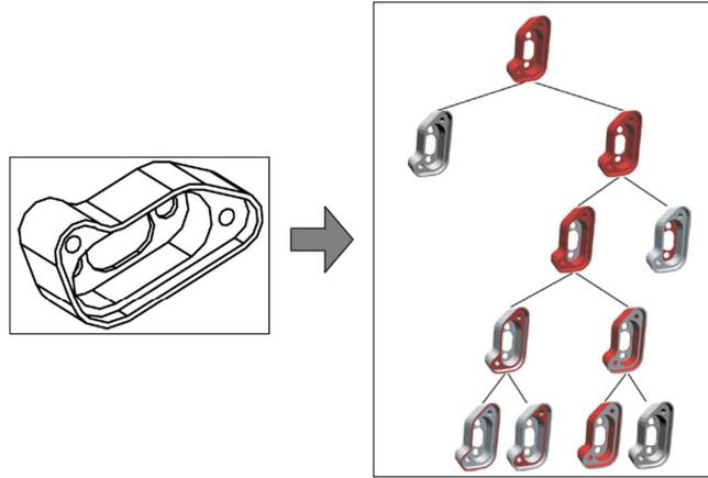
Figure 30: Scale-space decomposition of a mechanical part (Figures taken from [18] © 2006 Elsevier Ltd.).
