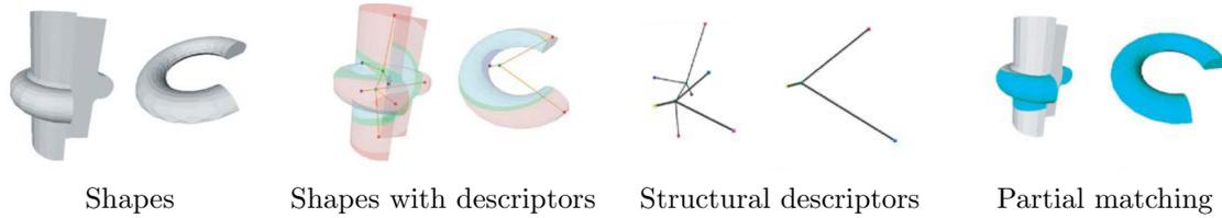
Figure 28: Sub-part correspondence of two mechanical parts (Figures taken from [23] © 2006 Elsevier Ltd.).
