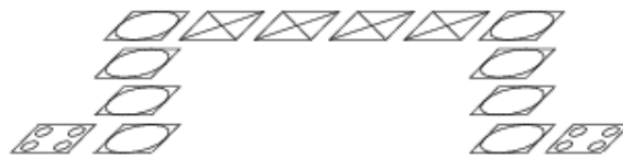
Figure 2.26: QCA cell style convention used to visually distinguish the cells on the Main Cell Layer from the cell used in via and crossover connections.
