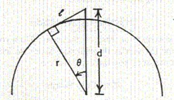
The required height is d - r, and since  $\cos \theta = r/d$ , we have  $d - r = (r/\cos \theta) - r$ . The hard part is to find  $\theta$ . If x = 3 feet is the length added the rope, then  $\ell$  must be the arc length  $r\theta$  plus .5x. This leads to
