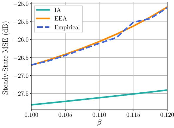
**Fig. 3** Steady-State MSE for the  $N = 2$  configuration. The empirical results were obtained by the usage of  $10^6$  independent Monte Carlo trials.
