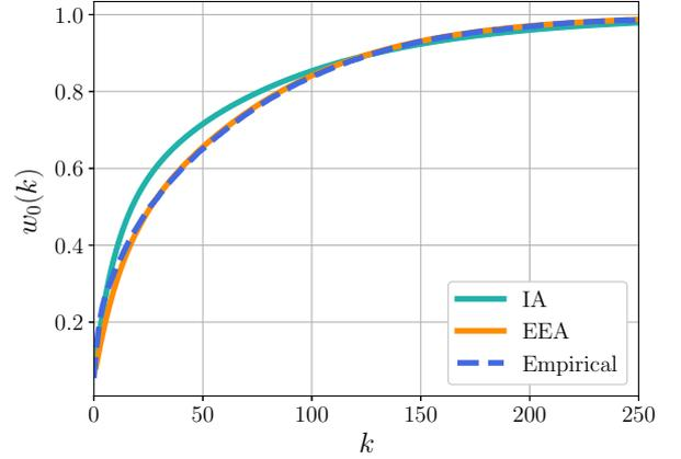
**Fig. 1** Evolution of the mean value of adaptive weight  $w_0(k)$  of the LMS with  $N = 6$  and  $\beta = 0.065$ . The empirical curve was obtained with  $10^7$  independent Monte Carlo trials.
