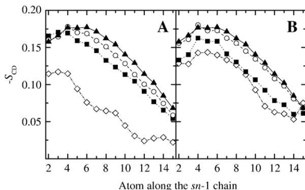
Fig. 6. Deuterium order parameter  $S_{CD}$  of DPPC *sn*-1 chains for different ranges of the distance  $R$  to the closest NBD-PC molecule in 4 C6-NBD-PC:60 DPPC (A) or 4 C12-NBD-PC:60 DPPC (B). Curves relative to  $R < 0.6$  nm (◇),  $0.6 \text{ nm} < R < 1.2$  nm (■), and  $R > 1.2$  nm (○) are shown, together with that obtained for pure, unperturbed DPPC (▲).
