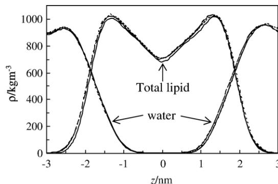
Fig. 7. Mass density profiles of water and total lipid as a function of transverse position relative to the center of the bilayer ( $z$ ) obtained in the simulations of pure DPPC (solid lines), 4 C6-NBD-PC (dashed lines) and 4 C12-NBD-PC (dotted lines).
