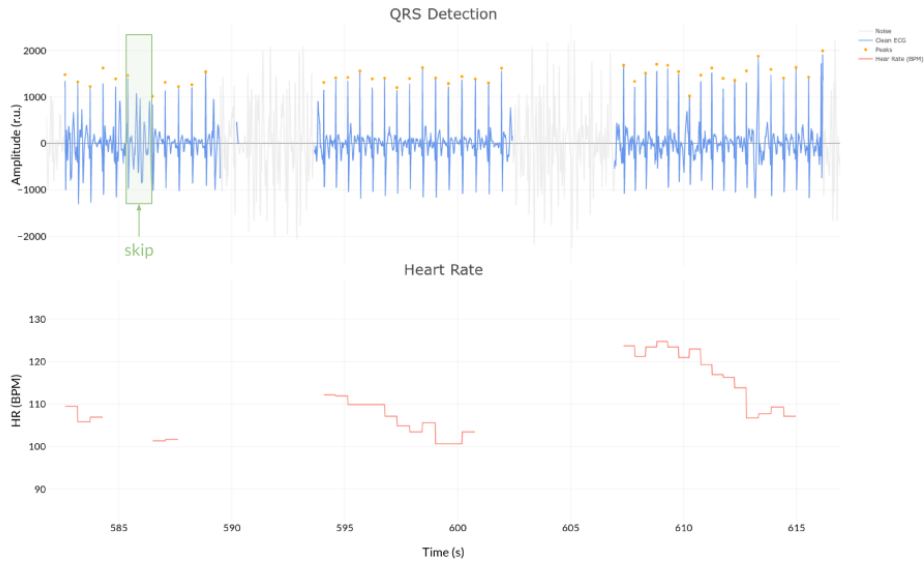
Figure 16: Heart Rate determination in the areas of clean ECG. The areas that are not represented in the Heart Rate plot are either noise or false peak detections.
