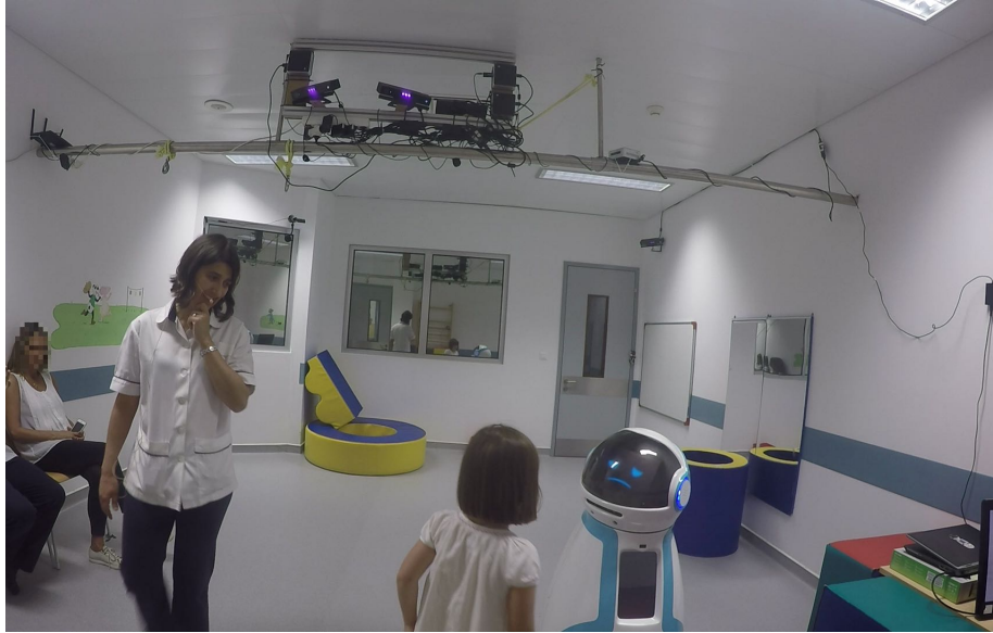
Figure 8: Example of a task specific behavior of the robot. Upon detecting an obstacle, ASTRO makes a sad face and tries to find a way around, before asking the child for assistance. In the background it is visible the whole hardware infrastructure of INSIDE.
