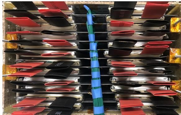
**Figure 5.1:** Cells, cooling plates and thermistors' cables top-view.
