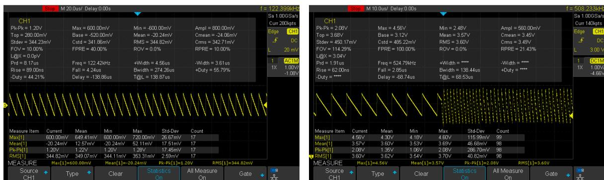
Figure 5.4:  $V_{REF1}$  signal measured with an oscilloscope.
