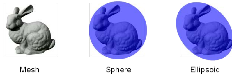
Figure 1.8 – Examples of bounding volumes that completely enclose a detailed mesh object.
