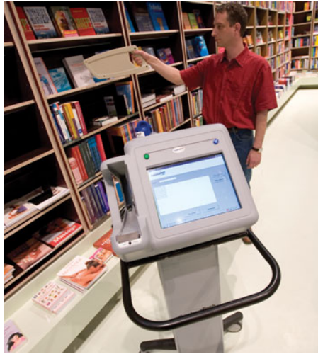
Figure 4.4: RFID Mobile Station - Source: http://www.mmh.com
