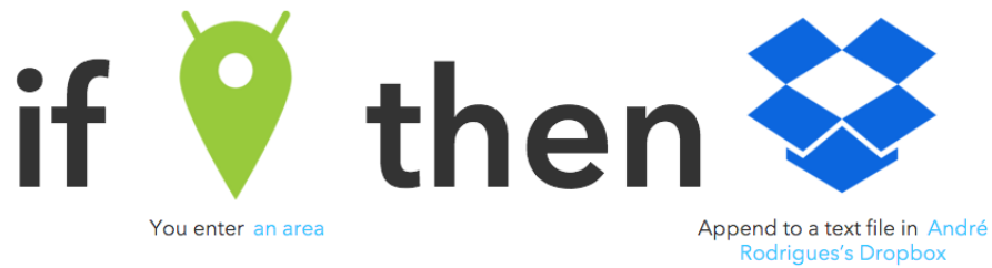
Figure 2.4: A rule in IFTTT that uses the Android Location and the Dropbox channels.
