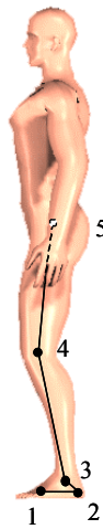
Figure 5.24: Kinematic structure of the analytical model. The results produced by this model are compared with the corresponding results produced by the multibody biomechanical model.
