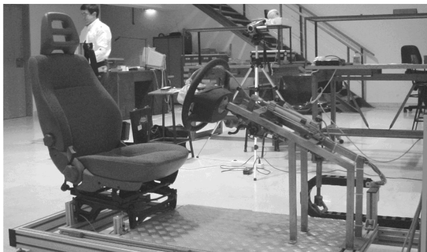
Figure 4.30: Vehicle seat used in the experimental setup to find the occupant initial conditions
