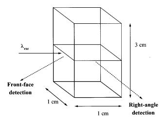
FIG. 1. Tridimensional cell showing the two experimental used detection geometries also reproduced in the MC simulation. The enclosure size and shape correspond to a typical fluorescence cell.
