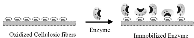
Fig. 4. Schematic representation of physical adsorption of lipase onto cellulosic fibers.
