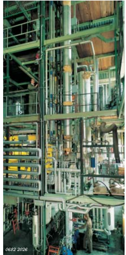
Multi-purpose pilot plant for the separation of mixtures by distillation, using Sulzer structured packings of various design.
