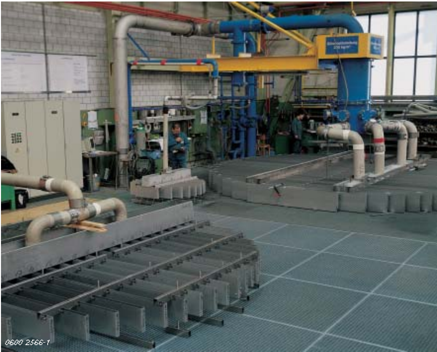
Distributors on the Sulzer Chemtech distributor test facility
