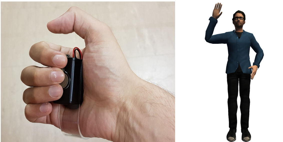
Figure 4.8: Our custom made device for tracking hand's rotation and its open / grab state (left) and users' avatar in our virtual environment (right).
