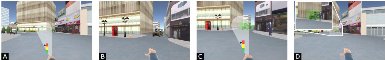
Figure 1: PRECIOUS technique for out-of-reach object selection: A) selection cone intersecting several objects, B) refinement phase, moving user closer to intersected objects, C) single object selection, D) returning to original position with object selected.
