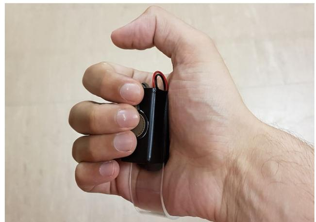
**Figure 7:** *Our custom made device for tracking hand’s rotation and its open / grab state.*
