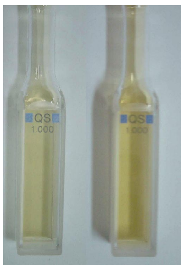
Figure 1. Visual appearance of a \text{NO}_2 + \text{N}_2\text{O}_4 mixture at 15 °C (left) and at 75 °C (right).
