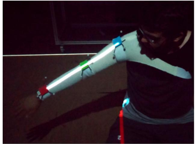
**Figure 2: Sleeve responsible for holding the tracking equipment.**
