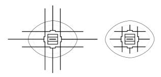
Figure 3. The length of the walls is computed by an intersection with the slab represented by a grey line.
