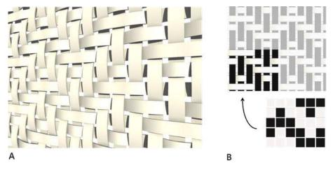
Fig. 6. A weaving movement created using the  $T_{weaved}$  algorithm: A. the obtained model in Rhinoceros 3D; B. the weaving pattern conceptual representation.
