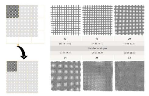
**Fig. 13.** On the left: Rationalization process of a weaving pattern. On the right: The application of the  $R_{weaved}$  algorithm – according to the number of stripes given, the algorithm returns the solution that is more affordable to fabricate.
