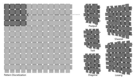
**Fig. 12.** Left: Discretization process of a façade weaving pattern based on a *piedpull* pattern; Right: a set of different façade modules resulting from different weaving patterns.
