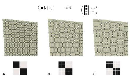
Fig. 7. Three weaving patterns available in the GS: A. chess, B. double-chess, and C. triple-chess.
