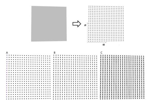
Fig. 2. Top: the surface discretization into a  $n \times m$  matrix of points. Bottom: the generation of vertical stripes – A. selection of a matrix' column; B. creation of a stripe axis at each column; C. generation of the stripes.
