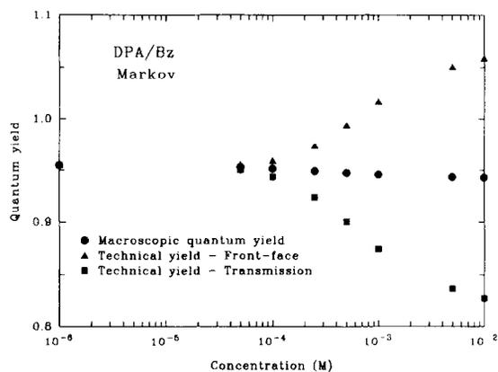
Fig. 11. Quantum yields of DPA solutions in benzene when excited at 337 nm: (●) macroscopic quantum yield; (▲) technical “quantum yield” for front-face geometry; (■) technical “quantum yield” for transmission geometry.
