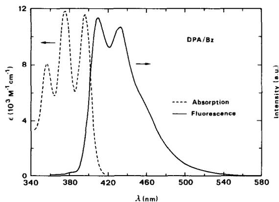
Fig. 1. Molecular fluorescence (—) and absorption (---) spectra of DPA in benzene.
