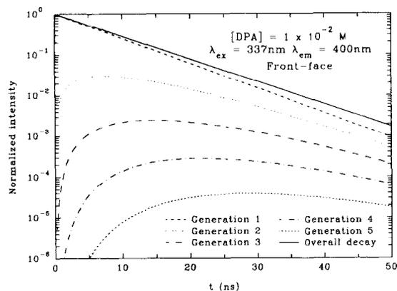
Fig. 5. Contribution of several generations of excited molecules to the overall observed decay observed at 400 nm for a  $10^{-2}$  M solution of DPA in benzene excited at 337 nm using front-face viewing: (---) 1st generation; (···) 2nd generation; (- · -) 3rd generation; (- · - ·) 4th generation; (- - - -) 5th generation; (—) overall decay curve. The overall decay includes the contribution of 15 generations of excited molecules.
