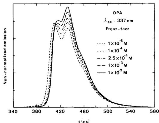
Fig. 9. Fluorescence spectra of several solutions of DPA in benzene excited at 337 nm using front-face viewing: (---)  $10^{-6}$  M; (···)  $10^{-4}$  M; (-·-)  $2.5 \times 10^{-4}$  M; (— — —)  $10^{-3}$  M; (—)  $10^{-2}$  M.
