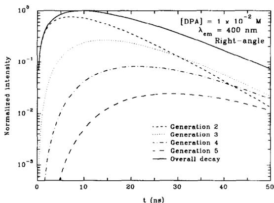
Fig. 7. Contribution of several generations of excited molecules to the overall observed decay observed at 400 nm for a  $10^{-2}$  M solution of DPA in benzene using front-face viewing: (---) 2nd generation; ( $\cdot \cdot \cdot$ ) 3rd generation; (-  $\cdot$  -) 4th generation; (— — —) 5th generation; (—) overall decay curve. The overall decay includes the contribution of 15 generations of excited molecules.
