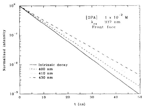
Fig. 6. Normalized decay curves of a  $10^{-2}$  M solution in benzene excited at 337 nm using front-face viewing for several emission wavelengths: (—) intrinsic decay curve; (---)  $\lambda_{em} = 400$  nm; (···)  $\lambda_{em} = 410$  nm; (- · - ·)  $\lambda_{em} = 430$  nm. The decays include the contribution of 15 generations of excited molecules.
