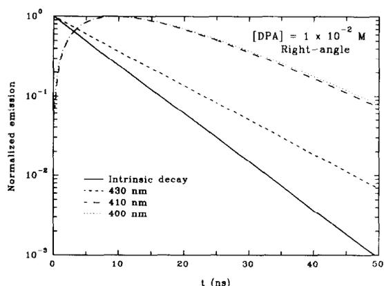
Fig. 8. Normalized decay curves of a  $10^{-2}$  M solution in benzene using right-angle viewing for several emission wavelengths: (—) intrinsic decay curve; ( $\cdot \cdot \cdot$ )  $\lambda_{em} = 400$  nm; (-  $\cdot$  -)  $\lambda_{em} = 410$  nm; (---)  $\lambda_{em} = 430$  nm. The decays include the contribution of 15 generations of excited molecules.
