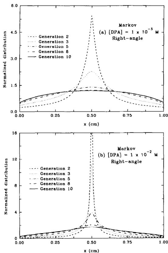
Fig. 4. Normalized distributions functions for several generations of excited molecules obtained by homogeneous Markov chains for (a)  $10^{-3}$  M and (b)  $10^{-2}$  M DPA solution in benzene using right-angle viewing geometry: (---) 2nd generation; (···) 3rd generation; (- · -) 5th generation; (- -) 8th generation; (—) 10th generation.
