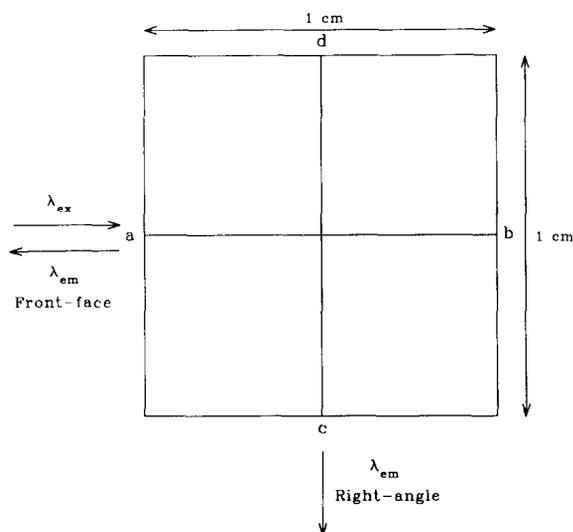
Scheme 2. The excitation/emission geometries considered in the unidimensional simulation and used to predict the fluorescence spectra and decay curves.
