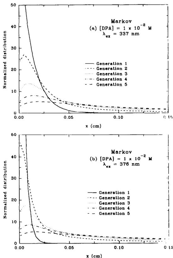
Fig. 3. Normalized distributions functions for several generations of excited molecules obtained by homogeneous Markov chains for  $10^{-2}$  M DPA solution in benzene excited at (a) 337 nm and (b) 376 nm using front-face viewing geometry: (—) 1st generation; (---) 2nd generation; (···) 3rd generation; (- · -) 4th generation; (- - -) 5th generation.
