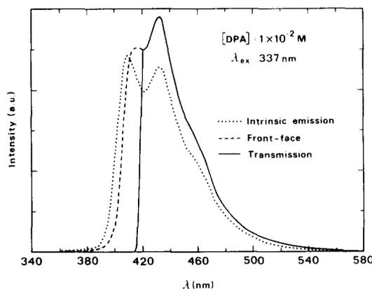
Fig. 10. Intrinsic fluorescence spectrum (···) and technical fluorescence spectra in front-face (---) and transmission (—) geometries for  $10^{-2}$  M solution of DPA in benzene excited at 337 nm.
