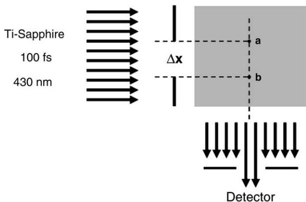
Fig. 1. Right angle geometry. The exciting radiation, with a flat intensity profile, passes through a slit  $\Delta x$ . The light scattered at point  $a$  has a delay  $\Delta x/v$  with respect to excitation light scattered at point  $b$ . Multiple scattering is not considered.
